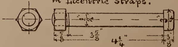
2-No. 514, Round Head Bolts. in Eccentric Straps.
